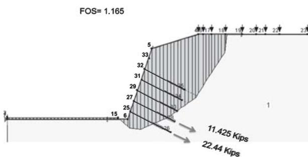
Figure 7. Failure surface with ground anchors
