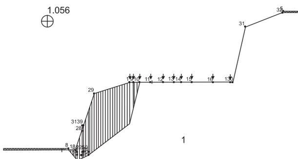
Figure 5. Failure slip surface with retaining wall
