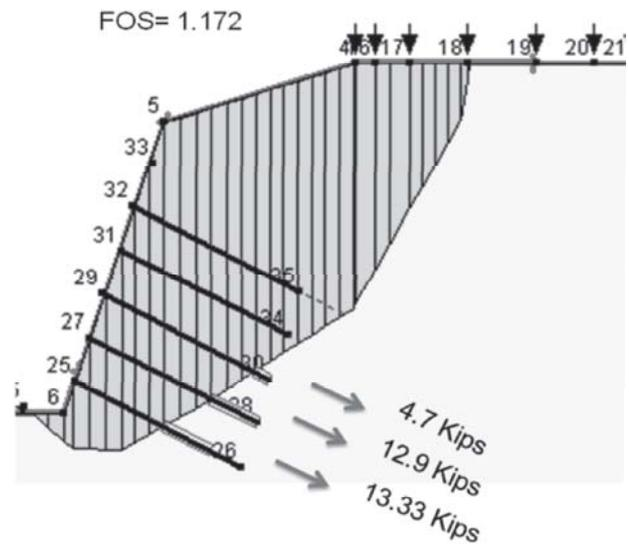
Figure 6. Slip surface with soil nails
