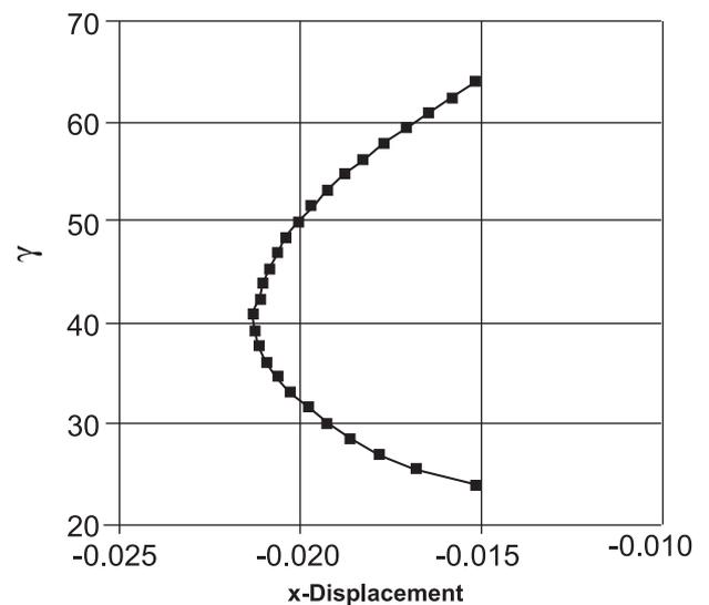
Figure 8. Displacement in horizontal direction in slope with Retaining wall
