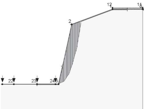
Figure 15. Failure surface of Slope 2
