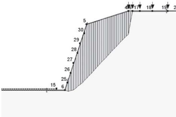
Figure 14. Failure surface of Slope 1
