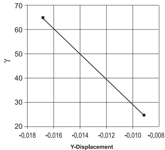
Figure 11. Displacement in vertical direction in slope with soil nails
