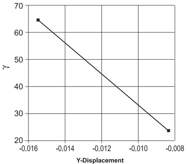
Figure 13. Y-Displacement in the slope with ground anchors
