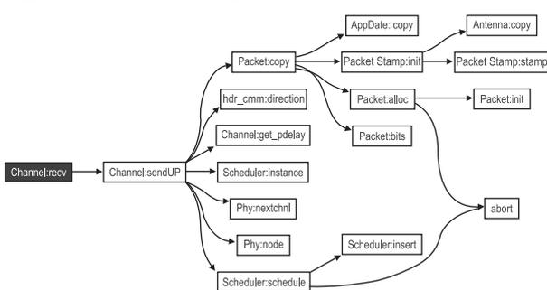
Figure 2. Receiver side implementation in NS-2 showing all the classes
