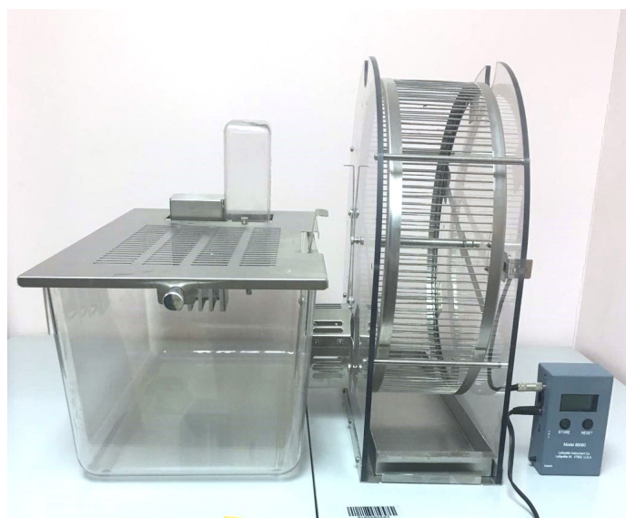
Figure 1: A cage equipped with voluntary rat running wheel with activity wheel counter.
