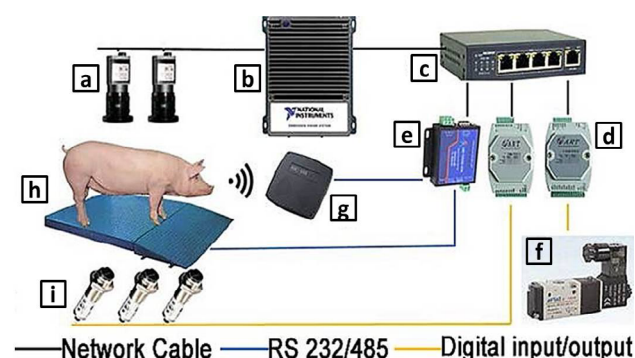
Fig. 2. The equipment in swine building of experimental station. a, binocular cameras; b, EVS-1463; c, Ethernet switch; d, digital input module; e, serial port server; f, pneumatic device; g, RFID reader; h, ground scale; i, photoelectric sensor.
