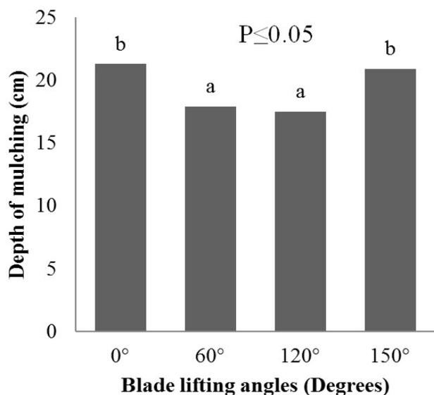
Figure 3: Effect of blade lifting angles on the depth of mulching.
