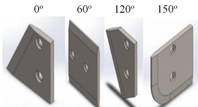
Figure 1: Blades with 0°, 60°, 120° and 150° lifting angles used for the comparison.
