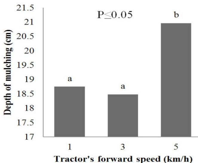
Figure 4: Effects of tractor's forward speed on the depth of mulching.
