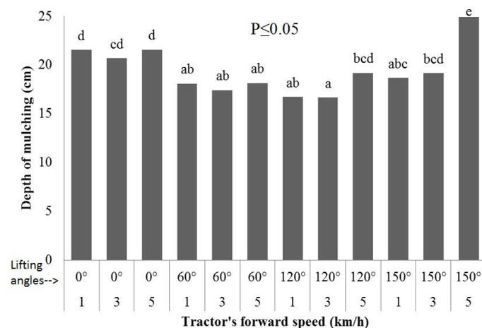
Figure 6: Effect of tractor's forward speed and blade lifting angles on the depth of mulching.
