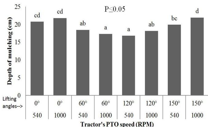
**Figure 7:** Effect of tractor's PTO speed and blade lifting angles on the depth of mulching.
