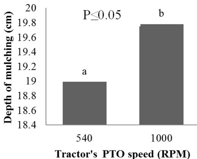
Figure 5: Effect of tractor's PTO speed on the depth of mulching.
