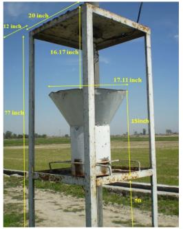
Figure 1: Schematic diagram of the light trap design.
