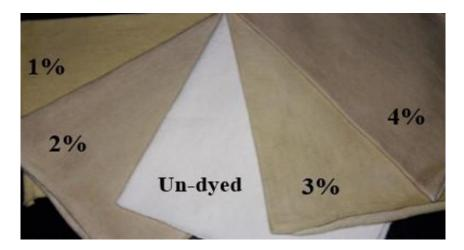
**Fig. 2.** Shade developed by varying fixing agent percentage and dyed under optimized dyeing time (120 min).
