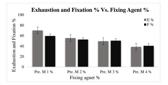
**Fig. 3.** Dye exhaustion and fixation percentage of dyed fabric by varying fixing agent percentage with 120 min dyeing time.
