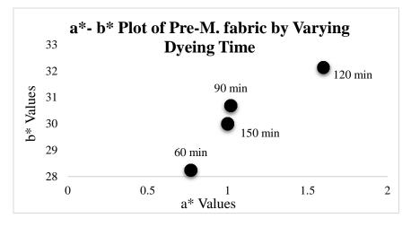
**Fig. 5.**  $a^*-b^*$  plot of pre-mordanted fabric using 1 percent fixing agent and varying dyeing time form 30, 90, 120 and 150 min.
