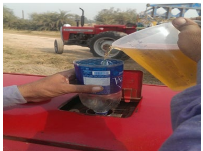
Figure 4: Measurement of fuel consumption
