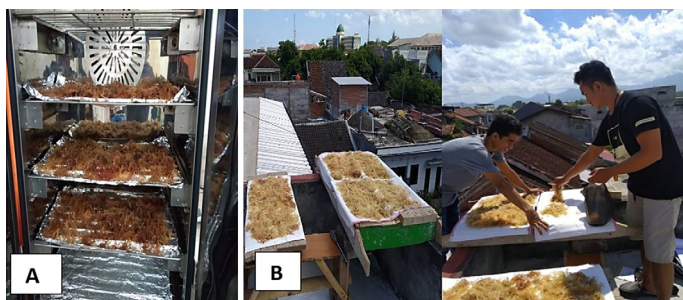
Figure 1: Cabinet dryer machine (A) and tray manual sun drying (B).
