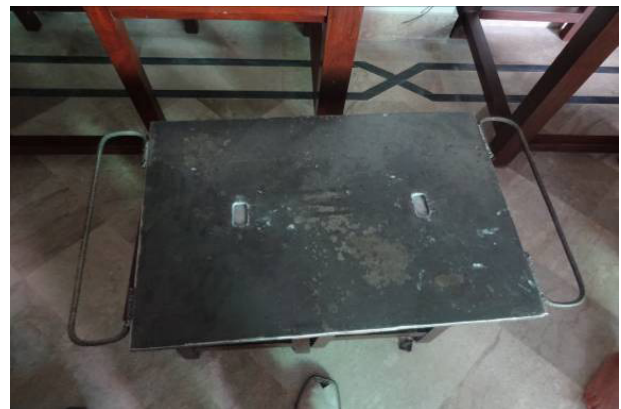
Figure 4: Load Cell showing grooves for installation of strain gauges
