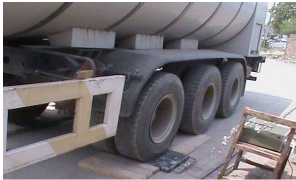
Figure 8: Axle wise weight of 4-axle truck while total weight being obtained at the same time from commercial weighing station
