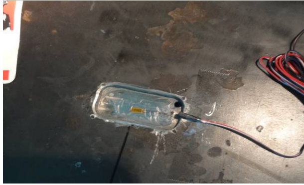
Figure 5: Strain gauge after installation on front side of Plate
