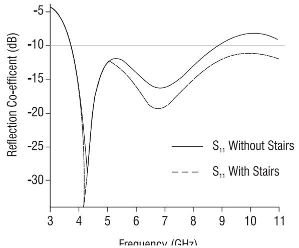
Fig. 3 Simulation result with and without stairs
