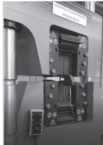
Fig 3. Instron 600DX Universal Testing Machine
