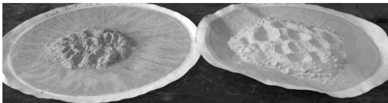
Figure 3: Products of Flotation, Concentrate (Right) and Tail (Left)
