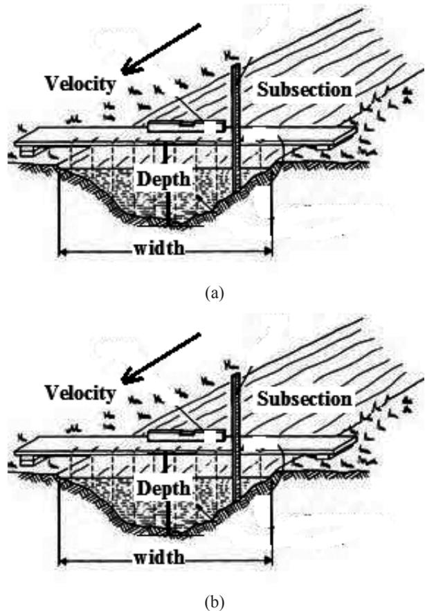
Figure 2: Illustration of methods of discharge measurement
