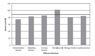
Figure. 2: Twelve hours noise level recorded at different zones of the Factory
