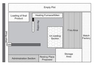
Figure 1: Layout of various zones in the Steel re-rolling mill
