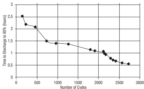
**Fig. 10: Time to discharge to 80% vs number of cycles**
