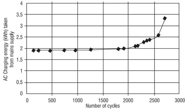
**Fig. 12: AC energy for charging the battery versus number of cycles**
