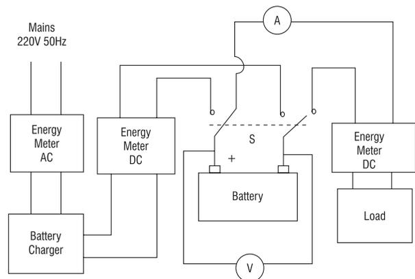
Fig. 9: Experimental set-up for finding the energy efficiency
