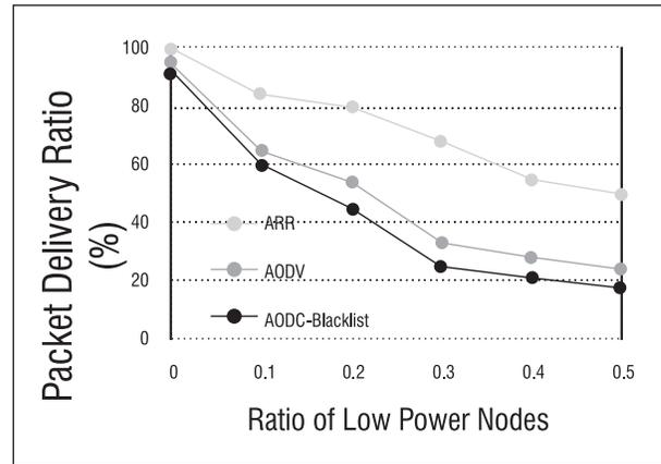
Fig. 2: Packet delivery ratio as a function of node power variables
