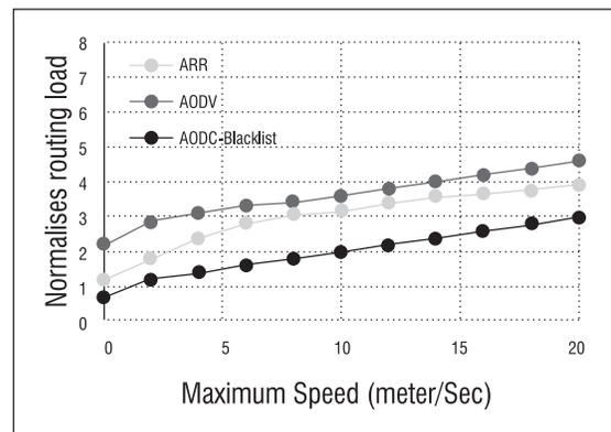
**Fig. 7: Normalized routing load as a function of mobility**
