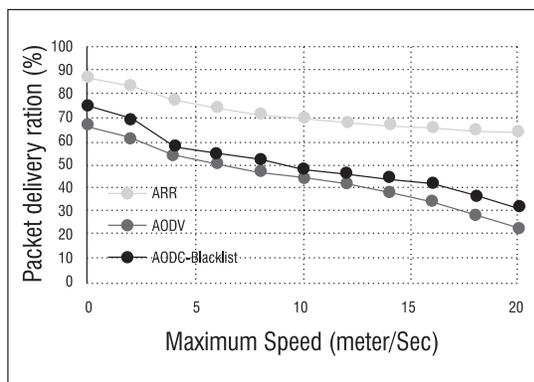
**Fig. 6: Packet delivery ratio as a function of mobility**
