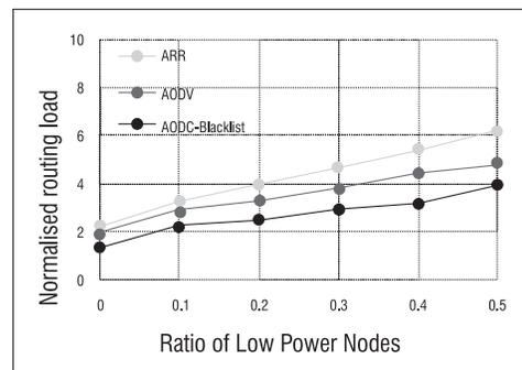
Fig. 3: Normalized routing load as a function of node power variables
