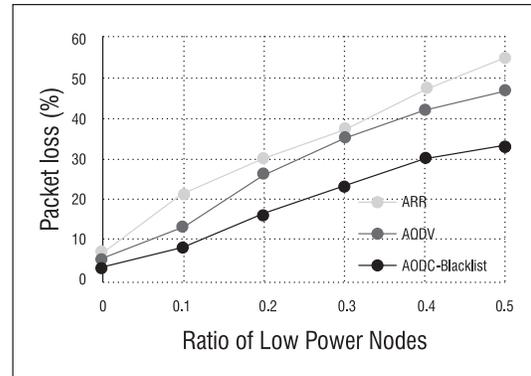
Fig. 4: Packet loss as a function of node power variables
