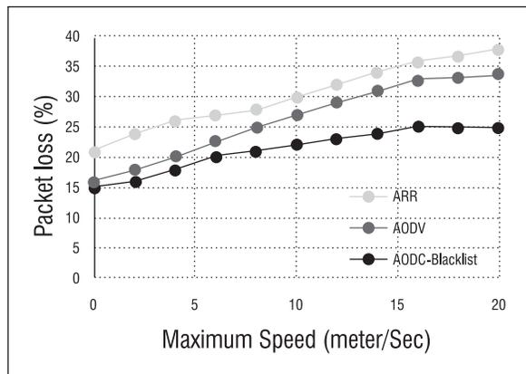
**Fig. 8: Packet loss as a function of mobility**
