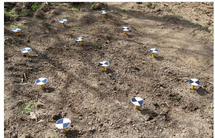
**Figure 3:** Erosion pipes installation in agricultural land.
