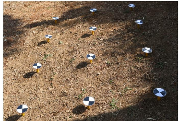
**Figure 2:** Erosion pipes installation in moderate forested area.
