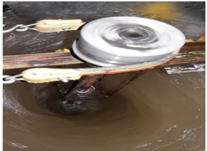
**Figure 6:** Vortex height and vortex formation at 0.004 m<sup>3</sup>/s.
