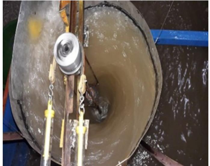
**Figure 5:** Vortex height and vortex formation at 0.7 m head.
