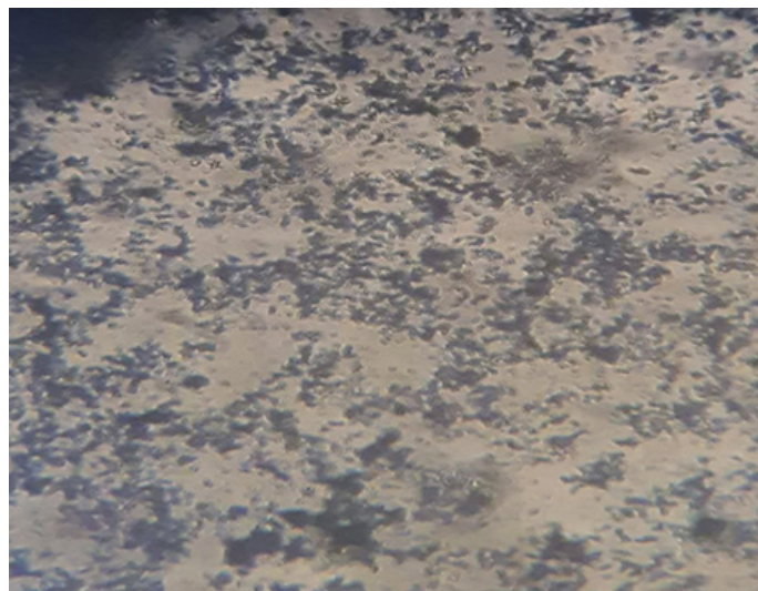
Figure 2: Micrograph of Cobalt Ferrite Nanoparticles (CoFe 2 O 4 NPs) by light microscope 100 x.
